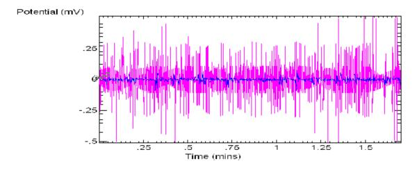
This plot is taken from a current and voltage noise test on tin in 1M NaCl. Shown in purple is the point to point voltage trace for the system not using a Noise Reducing Electrode and shown in blue is the same experiment using a Noise Reducing electrode. The use of a NR electrode allowed much finer features of the noise trace to be seen.
