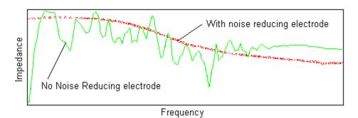
In the example above a working electrode of titanium is immersed in tap water with a lugin probe and SCE. Three electrode AC impedance was performed and the resulting Bode plot shown in green. For the second run using identical parameters a Noise Reducing electrode was added. The Bode plot is shown in red. It is apparent that the red curve is much smoother and because less averaging was needed by the instrument it was faster to obtain.
