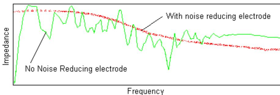
In the example above a working electrode of titanium is immersed in tap water with a lugin probe and SCE. Three electrode AC impedance was performed and the resulting Bode plot shown in green. For the second run using identical parameters a Noise Reducing electrode was added. The Bode plot is shown in red. It is apparent that the red curve is much smoother and because less averaging was needed by the instrument it was faster to obtain.
